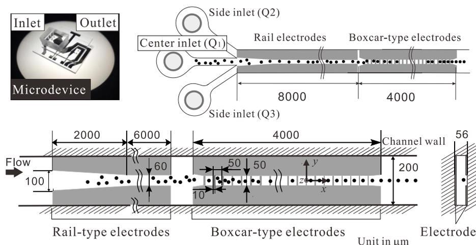
**Fig. 1** Photograph and schematic of the microchannel and boxcar-type electrodes.
