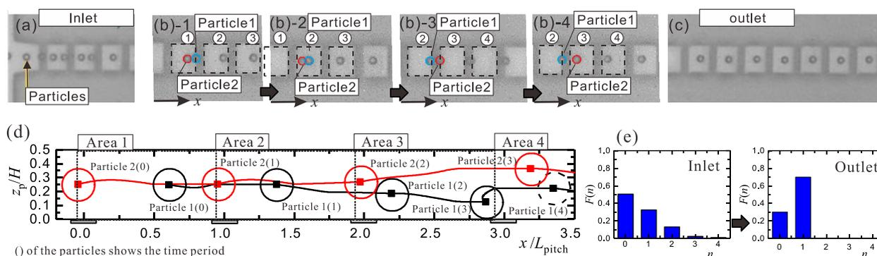
Fig. 2: (a) Photograph of particles at inlet of the boxcar-electrode region. (b) Snapshots of the two particles located in the same periodic area separating and align in the downstream region. Numbers shown over the boxes show the same spatial box. (c) Particles at outlet (aligned). (d) Motion trajectory of the two particles initially located in the same periodic region (computation). (e) Probability density function of the number of particles located in the same periodic region (period).
